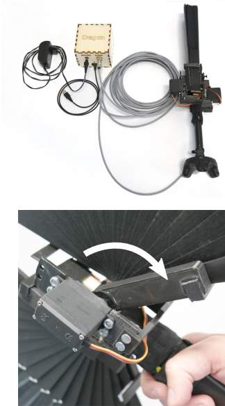
Figure 2: Top: The Drag:on is connected with a long cable to a box holding the microcontroller and circuits. Motor power is provided by an external power adapter. Bottom: A servo motor and connected arm opening a fan.
