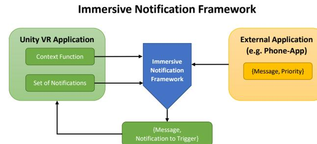
**Figure 3:** Conceptual architecture of the framework.
