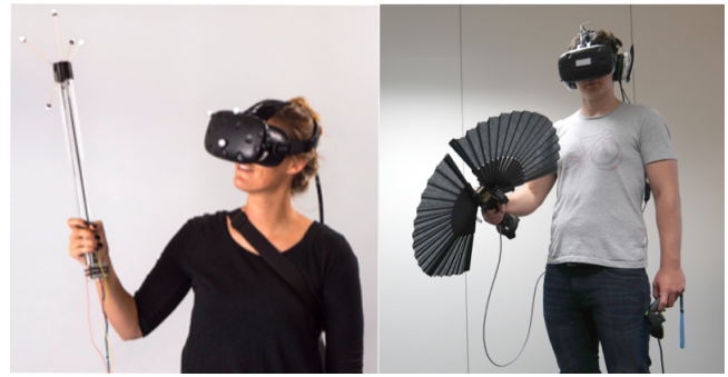
Figure 2: A great amount of past research efforts have concentrated on the development of specialized hardware, such as the haptic VR controllers Shifty [27] and Drag:on [28].
